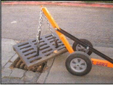
Grate Lifting Chain w/Steel Heavy Duty Dolly
