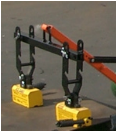
Twin Magnet Spreader Bar w/2 Heavy Duty Magnets
