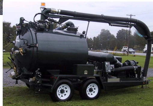
1000PD Trailer Mounted Vacuum Pumping System
