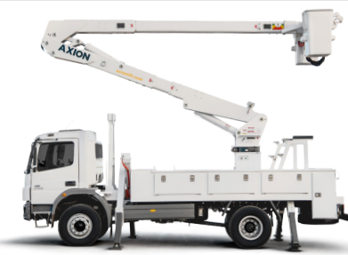
Serie AHN Working height: 49.2 ft to 65.9 ft 15,0 m to 20,0 m
