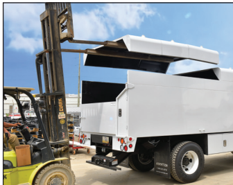
Lift rear sections off
