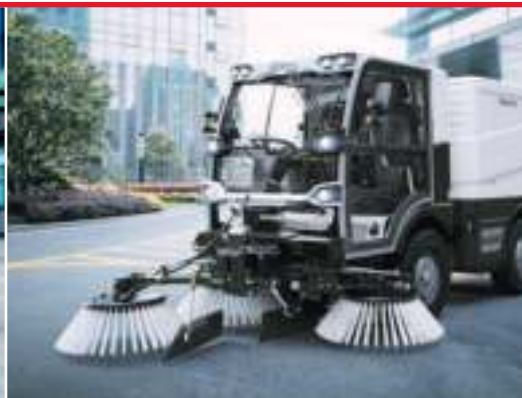
Pulled brush system with 3 rd brush
