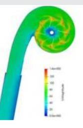
CFD State of the art CFD analysis assists in determining an airflow design of maximum efficiency for the entire system.
