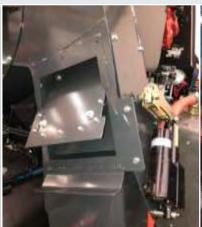
**Vacuum Enhancement Gate** The operator can vary the position of the actuator controlled by-pass gate to suit sweeping conditions and maximize performance.
