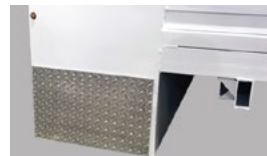
Tread Plate Rock Guards on Front Wall
