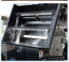
**HEAVY SWEEP PACKAGE** Elevator Type: 11 Flight squeegee with replaceable corded rubber tips; Continuous molded rubber belts and a Direct drive Hydraulic Motor: Optional **ELEVATOR WASH-OUT** System significantly reduces end of day cleaning for the operator.
