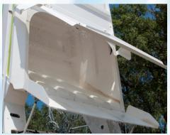
LARGEST HOPPER IN IT'S CLASS The Global M3 includes a 5.6 cu/yd hopper capacity compared to 3.5 cu/yd for competitive machines resulting in more curb miles swept between dump cycles. With near Full Useable Capacity, 12,000 Lift Capacity, and the Optional Hopper Wash Out System. Global M3 is Affordable, Reliable and Innovative.
