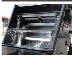
HEAVY SWEEP PACKAGE Elevator Type: Standard 11 Flight squeegee with replaceable corded rubber tips; Continuous molded rubber belts combine with standard Heavy Sweep Package make Global M4HSD the logical choice for sweeping heavy debris such as road millings, sand and gravel up to 3-tons per-minute. That Is one ton every 20 seconds! Standard leaf gate system assists in picking up large debris, bottles, large branches and leaves.
