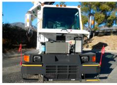
**ACCESS IT ALL** The **Global M4HSD** features many maintenance-friendly attributes, such as a rear swing-out radiator, easy access front mounted AC condenser, brake and windshield washer fluid reservoirs, and cab fresh air filter.
