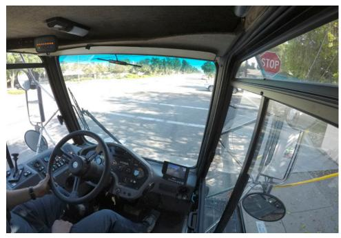
The inherent design of the **Global M4HSD** makes it the logical choice among heavy-duty mechanical sweepers. With the center mounted/cab forward layout the operator has unsurpassed visibility of the road surface as well as pedestrians and surrounding traffic. The large hopper capacity equals more lane miles swept between dump cycles and the **18.5' turning radius** makes the **Global M4HSD** highly efficient and comfortable.
