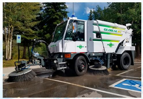
THREE POWERFUL BROOMS Optional Front Articulating brush allows for extra reach to shoulders and center islands. Via In-cab joystick, the articulating front brush can be positioned on left or right side allowing for sweeping on right or left without changing seating positions.
