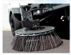
POWERFUL GUTTERBROOMS Large 47" Digger-Type Gutterbrooms allow for superb cleaning of curbs and help guide the debris to the 72" wide Pick Up Hood. Combined with a Large 32" Suction fan equals one of the most powerful AIR Street Sweepers available today.
