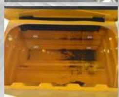
Global M3EV includes a 5.6 cu/yd hopper capacity compared to 4.5 culyd for competitive machines resulting in more curb miles swept between dump cycles. With near Full Useable Capacity, 12,000 Lift Capacity, and the Optional Elevator and Hopper Wash Out System, Global M3EV is Affordable, Reliable and Innovative.
