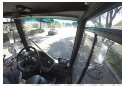
The inherent design of the Global M4EV makes it the only choice among 4-wheel mechanical sweepers. With the center mounted/cab forward layout the operator has unsurpassed visibility of the road surface as well as pedestrians and surrounding traffic. The large hopper capacity equals more lane miles swept between dump cycles and the 18.5-foot turning radius makes the **Global M4EV** highly efficient and comfortable.
