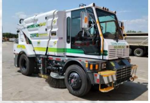
With travel speed of 55-MPH and a battery operational range of up to 8-hours, towns, villages and large cities will be able to clean the streets while protecting our environment and building a cleaner future with ZERO EMISSIONS. At the end of the shift just plug in the sweeper, recharge the batteries and sweep again.
