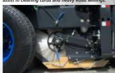
includes 280 Gallon Water Tank Capacity combined with Two(2) Diaphragm Water pumps and Two(2) Modes (LOW/ HIGH) provide versatility and superb dust control.
