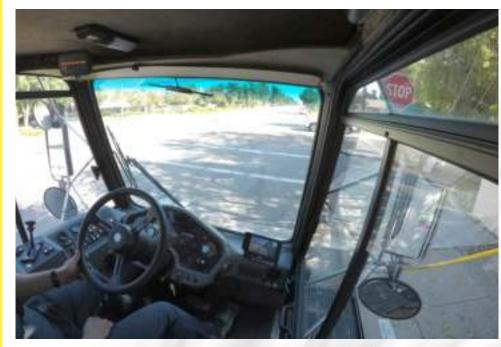
THE BEST TURNING RADIUS & EXCEPTIONAL VISIBILITY With the center mounted cab/forward layout the operator has unsurpassed visibility of the road surface as well as pedestrians and surrounding traffic. The 116-inch wheelbase allows for the sweeper to reach a turning radius of 12 1/2', wall-to-wall. With the pickup Head in the center you don't have to worry about what is happening behind you. The Global R3AIR EV's exceptional visibility increases operator and pedestrian safety.
