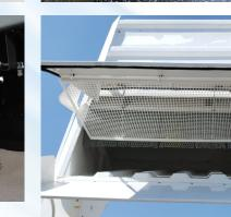
LARGEST HOPPER IN IT'S CLASS Global R4AIR includes a 5.8 cu/yd 100% Stainless Steel hopper construction, Cyclone Type Dust Separators and Swing-Down Hopper Screens are easy to clean.
