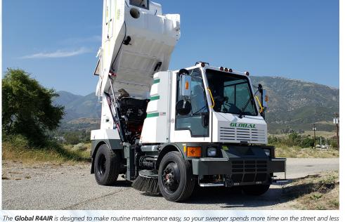
time in the garage. Two swing-out center body panels provide unrestricted access to Fan Housing, maintenance and daily cleaning. A centralized, weather-proof systems locker fully protects electrical components from the elements while fender located Hydraulic system allows for easy maintenance, accessibility and inspection. Troubleshooting is now a breeze.
