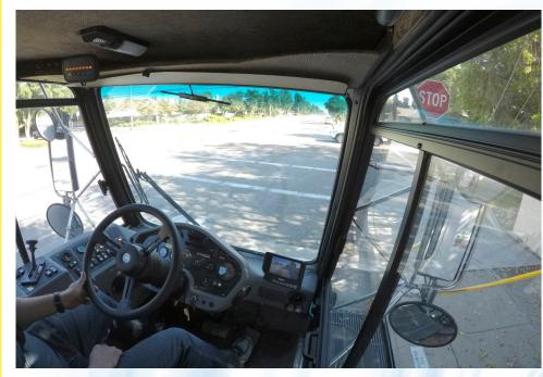
THE BEST TURNING RADIUS & EXCEPTIONAL VISIBILITY With the center mounted cab/forward layout the operator has unsurpassed visibility of the road surface as well as pedestrians and surrounding traffic. The 130-inch wheelbase allows for the sweeper to reach a turning radius of 18 1/2', wall-to-wall. With the pickup Head in the center you don't have to worry about what is happening behind you. The Global R4AIR's exceptional visibility increases operator and pedestrian safety.
