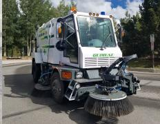
**Our 47-Inch Front Articulating Broom** is hydraulically controlled, retracts/extends, lowers/raises with additional four-way Gutterbroom tilt. All broom functions are controlled via Joystick located in the cab. The sweeping Path is extended to 139 Inches. Great for digging out curbs during heavy sweeping, and for tight cul-de-sacs and hard to reach areas.
