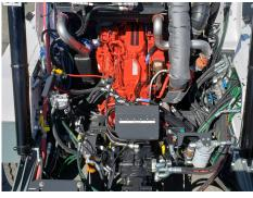
The Global R4AIR comes standard with a fuel-efficien Tier 4 Final, 6-cylinder, turbocharged 280-horsepower 6.7-liter Cummins ISB diesel engine, largest in its class, delivering outstanding performance and reliability.
