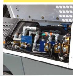
IT'S ALL IN THE OPEN Hydraulic Hoses are NOT hidden in the frame of the sweeper, while all Manifolds and Filters are located in a central location
