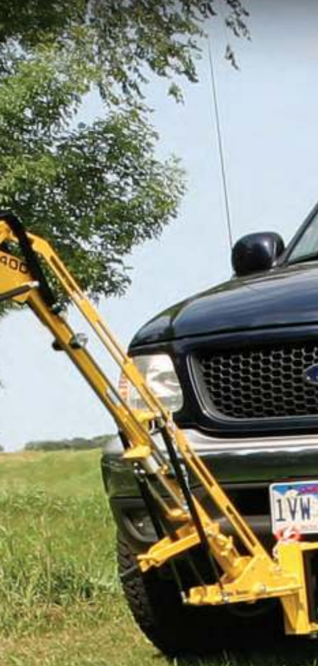
Flexible boom and tilting head for easily accessing valves that aren't perfectly straight.
