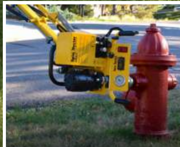
Optional 90° tilt to remove stubborn hydrant caps.
