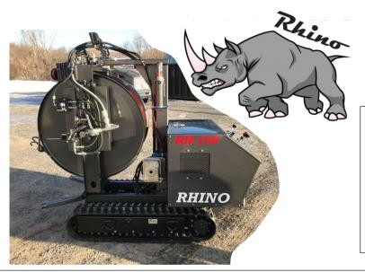
The Rhino Easement Reel is a powerful, self contained mobile reel crawler that allows remote operation of your sewer jetting equipment in otherwise unreachable areas. The machine is powered by a Gasoline engine and is drive by a hydrostatic drive system. The rubber track, variable speed and directional controls make the machine easy to maneuver on any terrain. The hose reel is powered In and Out and has variable speed controls.
