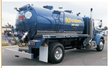
Single Axle Steel tanks up to 2500 Gallons, Aluminum Tanks up to 2800 Gallons
