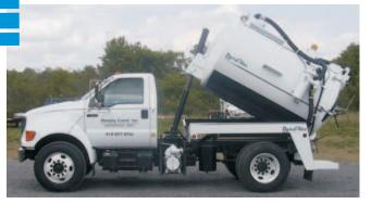
High Vacuum Industrial Use Vacuum Trucks, Clean Catch Basins, Sewers, Pits or any hard to move material
