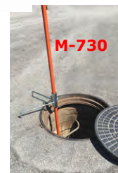
1) Place hose in jaws 2) Close Jaws around hose 3) Lower the guide into place 4) Pull rope and release hose and nozzle
