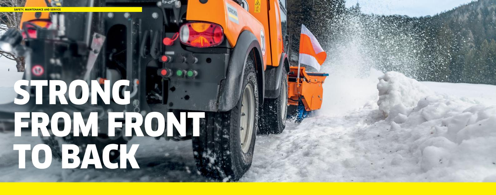
The Holder C 70 delivers high power in a small package. The power comes from a Kubota 4-cylinder diesel engine that supplies 65 HP (48 kW) power and meets the requirements of the Tier 4 Final exhaust emissions standard. The hydro-static traction drive over 4 wheel motors ensures sensitive and continuously variable speed regulation. When the machine is put to work, the electronic load limit con-trol automatically regulates the driving speed, ensuring that tasks are relaxed and effortless.
